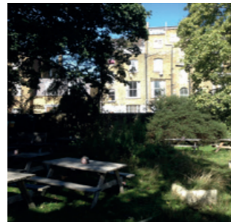
Rear elevation of nineteenth century terraced dwellings on the A24; proposed massing will need to avoid significant infringement to daylight, sunlight and rights to light. Proposed windows will need to be 18 or 20 metres away from existing windows to demonstrate that there will be no unacceptable loss of privacy. Where new apartments overlook existing gardens, privacy may also need to be carefully considered. The foreground comprises an area of green landscaping with mature trees. The outlook to these trees may be considered valuable to both the college and to neighbours.
