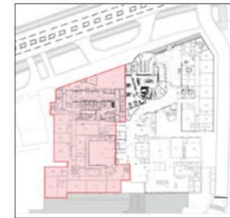
In addition to the areas noted above, option 3 includes part demolition of the 4-storey Block C, as far as the stairs to the Executive's office. It should be noted that this block also has a basement which contains the boiler house which has recently been totally replaced and services all of the elements of the Lambeth College site - including the 1950s, new frontage building on Clapham Common and the recently completed 4,000m 2 building at the rear of the site. We anticipate that the costs of replacing the boiler and associated facilities if this element was redeveloped would be in the order of £750,000 to £1m including building works.
